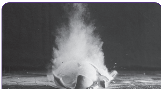
A rubber ball that has been frozen to near absolute zero by liquid helium
