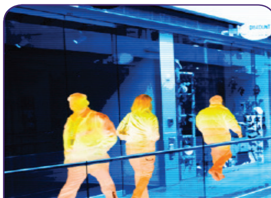
Infrared light is given off by warm objects such as human beings
